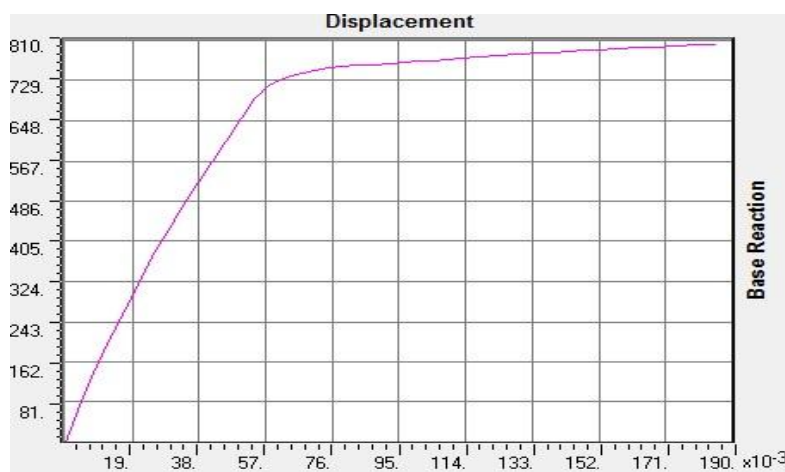
Figure 3. Showing Pushover Curve of a without infill wall frame in X direction
