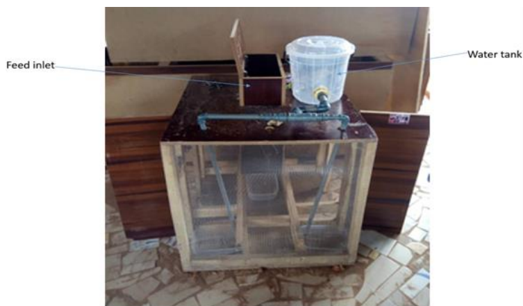
Fig. 9. The prototype of the automated feeding system for poultry farms
