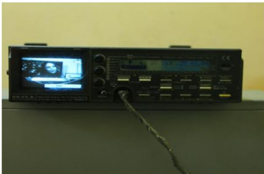
Fig. 2: Field strength meter(CATV)
