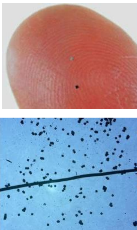
FIG-3 Hitachi powder-type tiny RFID tags (in contrast with a human hair) with a 128-bit of read-only memory and a size of 0.05mm × 0.05mm × 0.005mm
