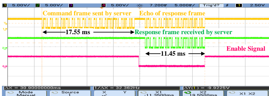
Figure 10: Command frame, response frame and Enable signals for Exception Responses
