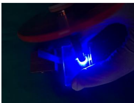
FIGURE-1 Preparation of nano-hybrid composite test specimen using a split metal mould
