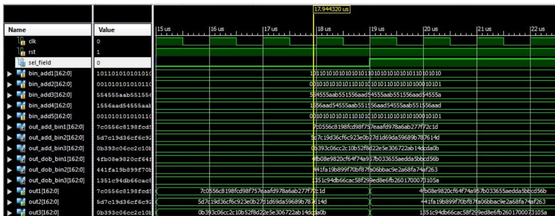
Fig 26. Simulation waveform of Point Addition and Point Doubling for 163 bits
