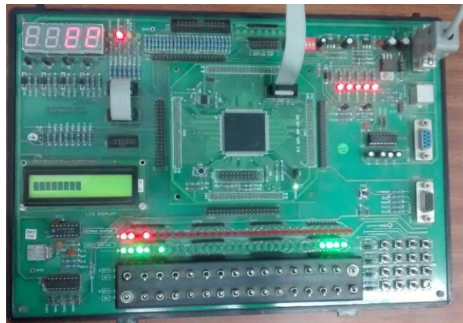
Fig 8. Hardware Implementation of the RSA Processor
