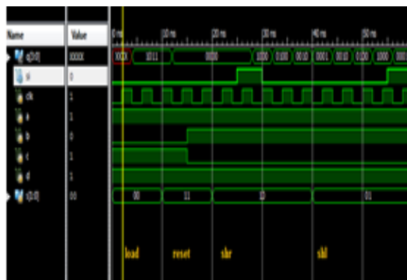
Figure 9: Simulation result of 4-bit universal shift register
