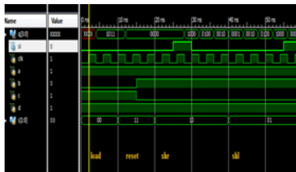
Figure 10: Simulation result of 4-bit universal shift register
