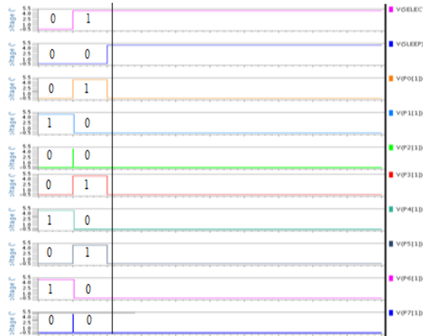
Fig.8: Simulated waveforms of IP Shifter using MTNCL
