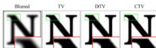
Fig. 4 Non-blind de-blurring of character ‘N’ using TV, DTV, CTV.
