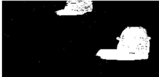
Fig. 5. Noisy binary mask result after GMM based background subtraction
