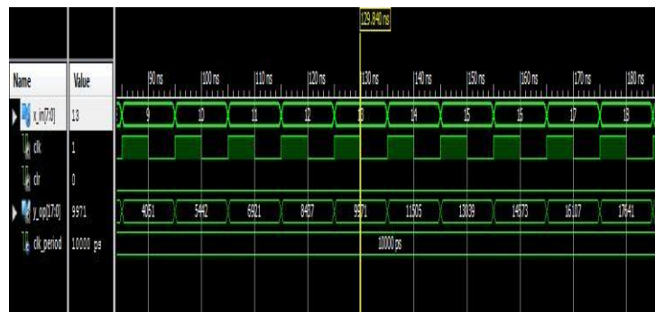
Fig.9: Simulation waveform for 12 Tap concurrent FIR filter
