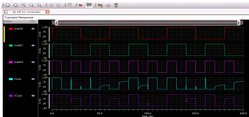
Fig 10 Simulated output of Modified GDI Full Adder
