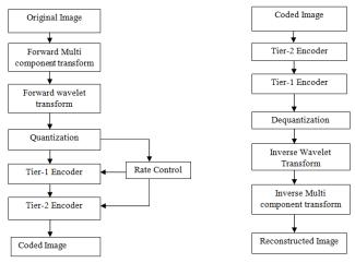
Fig.2 Original image to Coded image conversion Fig.3 Coded image to reconstructed image conversion
