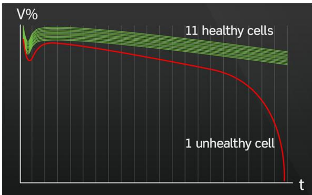
Figure 5: Battery cabinet discharge profile in view of a failed cell
