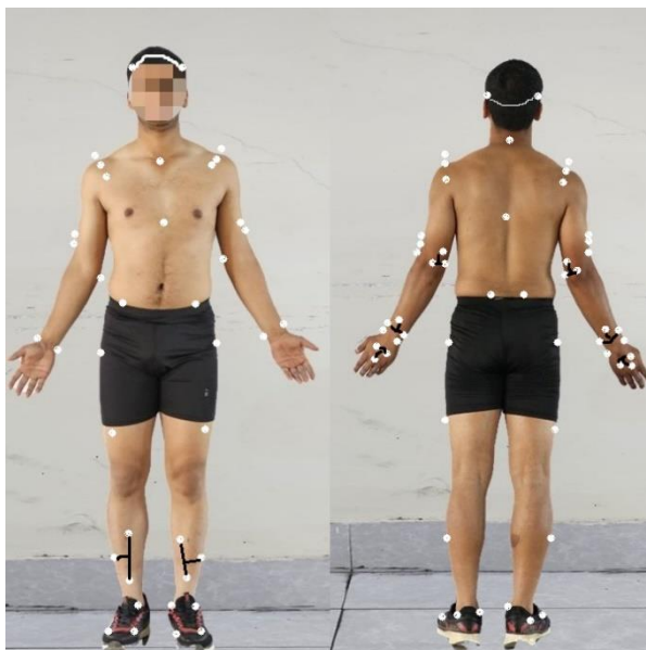
Figure 2. Custom marker sites on one participant's body while in anatomical standing position.
