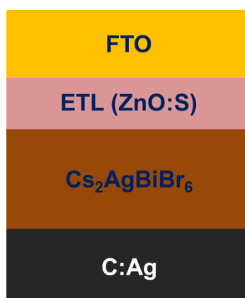
Fig. 3: Shows a conventional solar cell
