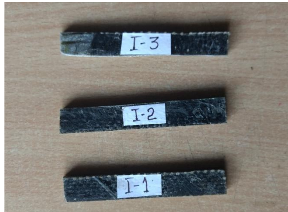
Fig. 2&3 Tensile and impact test samples
