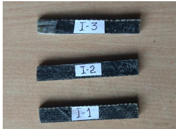
Fig. 2&3 Tensile and impact test samples
