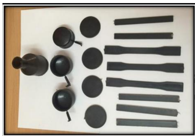
Figure 15: Moulded product of Rose petals Composite
