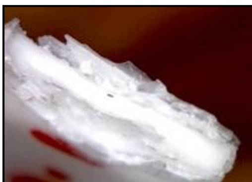
FIG.3: Fracture appearance of PC/TPU blend using optical microscope at -20°C
