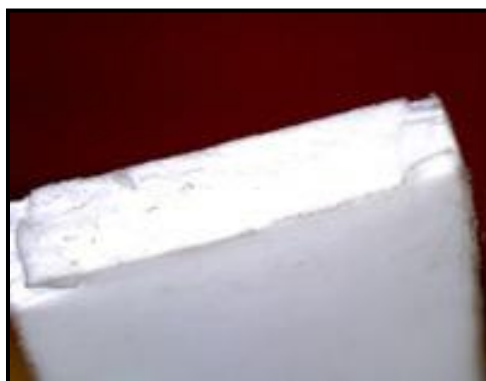
FIG.2: Fracture appearance of polycarbonate using optical microscope at -20°C
