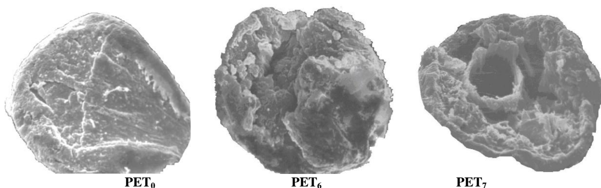
Fig. 8 SEM Scans of fractured FR PET fibres
