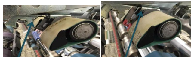
(A) (B) Fig.6. Old spring (A) and new spring (B).
