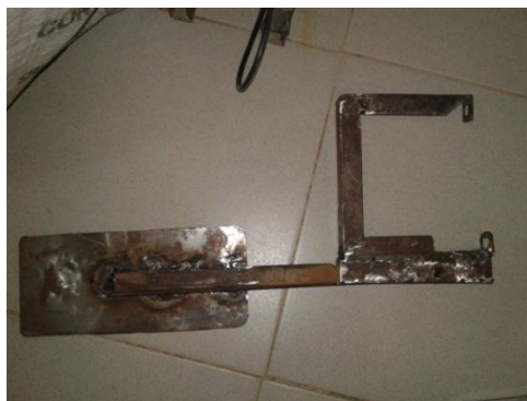
Figure 4: Tail (wind direction) welded with Frame
