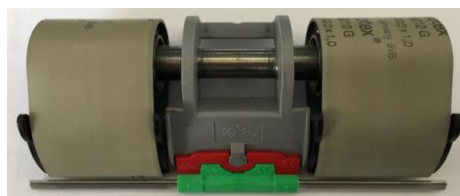
Fig.3. Active Cradle with roller, top apron, clip and pressure bar.
