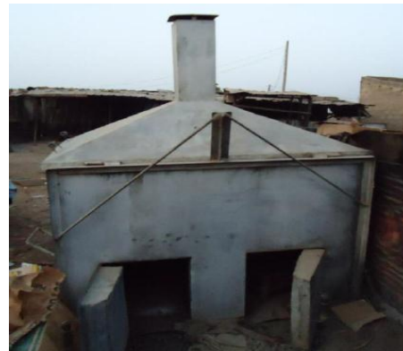
Fig. Fabricated smoking kiln with chimney
