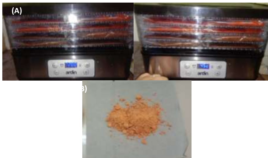
Figure III. 4 A) The process of drying kimchi using a Food Dehydrator ARD-PM99 at 45 °C for 72 hours; (B) Drying powder.
