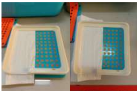
Figure III. 7 The process of filling capsule shells no. 0 using a semi-automatic capsule filling tool.
