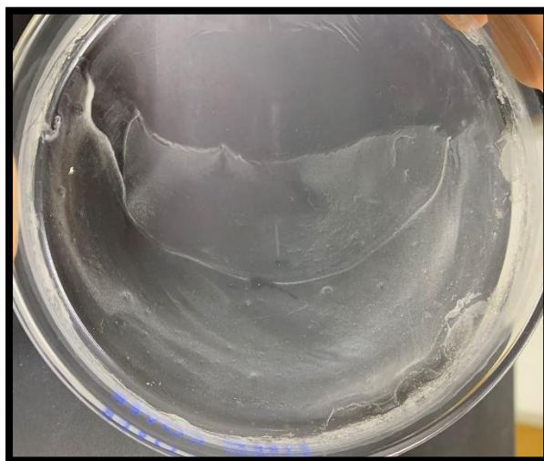
Figure 8. Polyhydroxybutyrate (PHB) sheet from the bacterial isolates NM17
