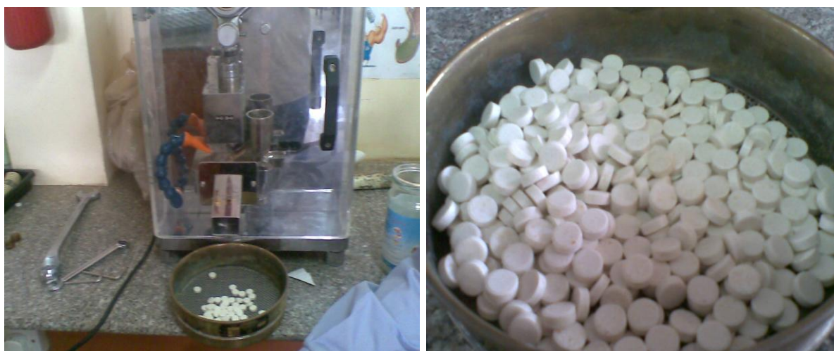
Figure 4. Tableting process of effervescent ciprofloxacin HCl
