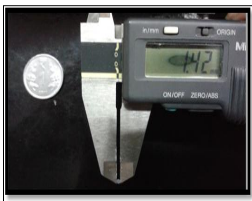
Fig 3. Measurement of the bead
