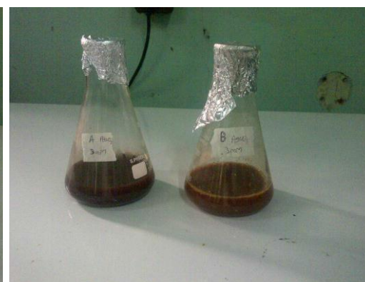
Fig 3a and 3b : Colour (brown) of the reaction mixture of 3mM silver nitrate, C. esculentus and B. paradoxum (B) seed extracts after 7 hours
