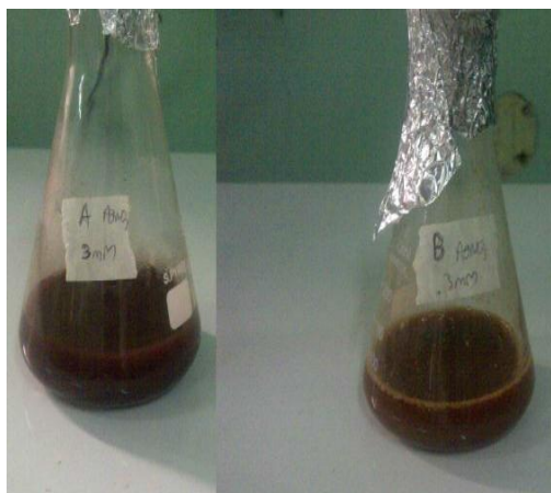
Fig 4a: Colour (dark brown) of the reaction mixture of 3mM silver nitrate and Cyperus esculentus (A) nitrate and Butyrospermum paradoxum (B) seed extracts after 24 hours
