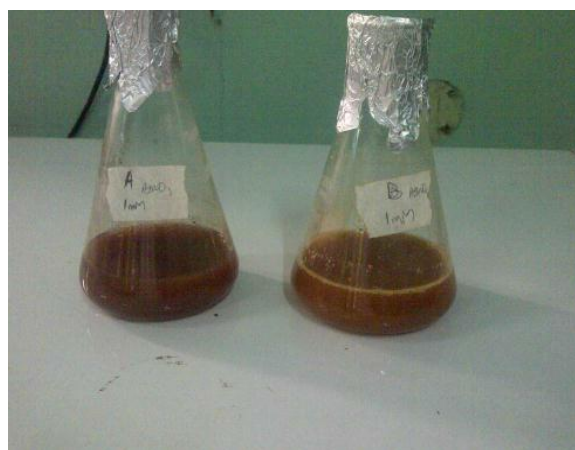
Fig 4b: Colour (brown) of the reaction mixture of 1mM silver nitrate, C. esculentus (A) and B. paradoxum (B) seed extracts after 24 hours.
