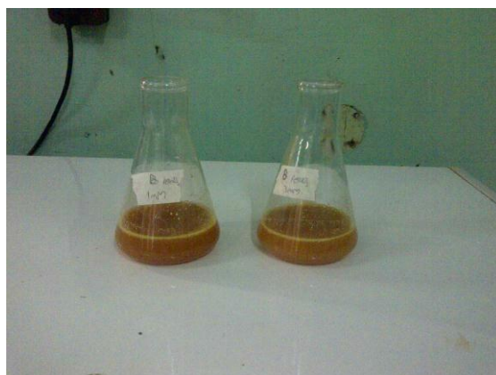
Fig 2 b: Colour (brown) of the reaction mixture of 1mM and 3mM silver nitrate and B. paradoxum seed extracts after 0 hour
