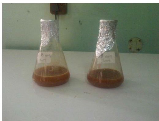
Fig 3a and 3b : Colour (brown) of the reaction mixture of 3mM silver nitrate, C. esculentus and B. paradoxum (B) seed extracts after 7 hours
