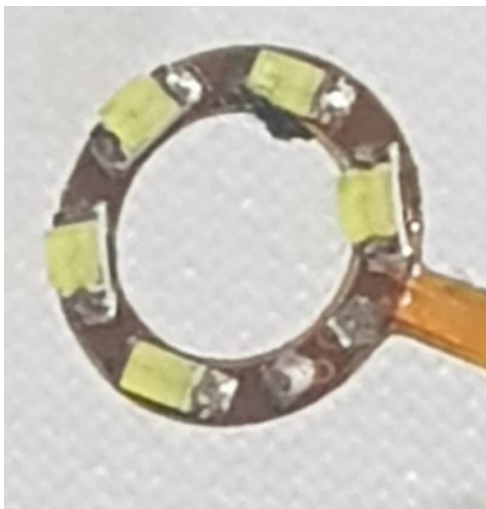
Fig 3. Assembly of five bright white light LEDs mounted on circular PCB.
