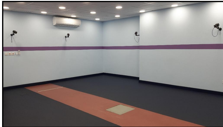
Figure (1): Eight-camera Vicon motion analysis system for 3 D gait analysis.
