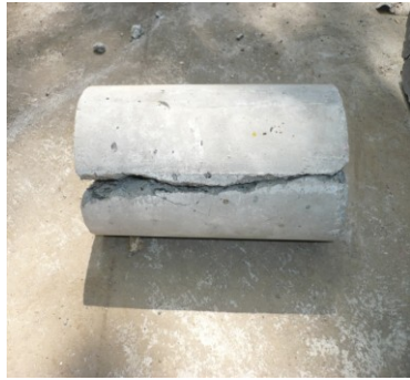
a) Conventional concrete Fractured into two pieces (b) Specimen reinforced with fibre Fig. 2 Crack pattern of cylinder
