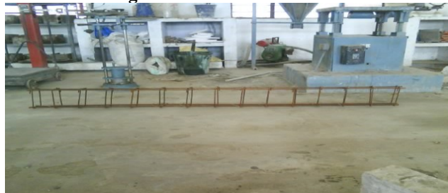
Fig 2.5 Reinforcement for Flexure Beam
