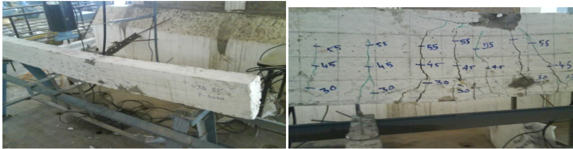
Fig 2.33 Crack Pattern of Flexural Beam
