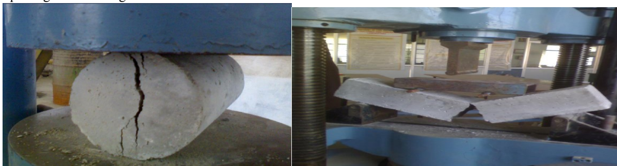
Fig 2.3 Split Tensile Strength of Cylinder & Flexural Strength of Beams
