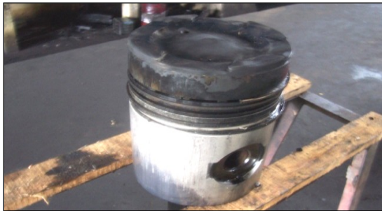
Figure 9. Piston ring broken
