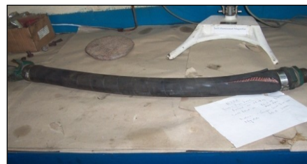
Figure.8 Flexible hose burst
