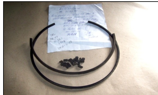
Figure10. Piston ring broken
