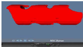
Fig.27 Iteration 4: Sloshing of LPG in a tank with two modified baffle showing peak amplitude of fluid
