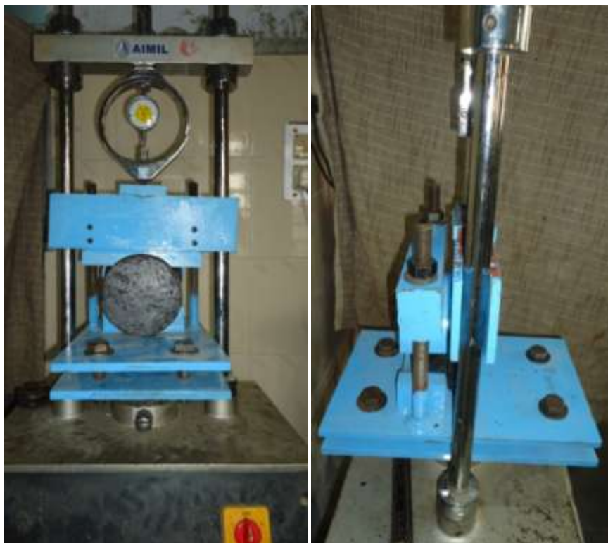
Figure 2.1: Schematic diagram and photographic view of the Shear-Testing Device.
