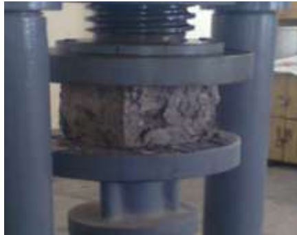
Fig. 3. Compressive Strength Test
