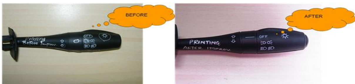
Figure 18 Scratches on printed symbol is corrected by monitoring of baking time and curing time and temperature.
