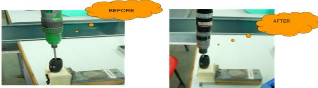
Figure 21 Tool correction made for increase in spring box hole diameter
