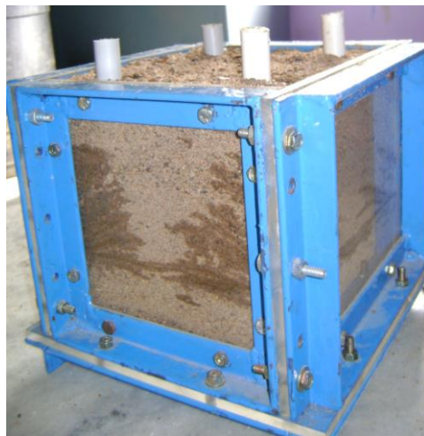
Fig. 2 Tank set up after the grout
