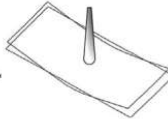
Figure 7: Predicted part warpage for centre-gated part
