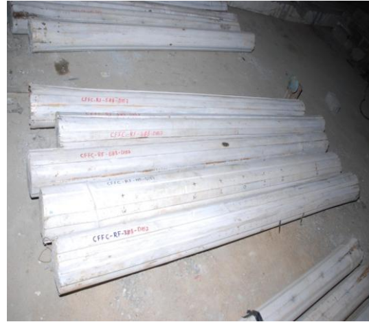
4 (b). Failure of columns at edges for L/D 15
