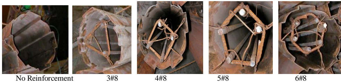
Fig 2.1. Rectangular fluted steel tube with and without reinforcement
