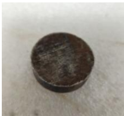
Figure 1. EN31 workpiece (solid cylinder, \varnothing 30.3 mm)
