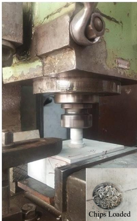
Fig.2. FSE process setup on milling machine
