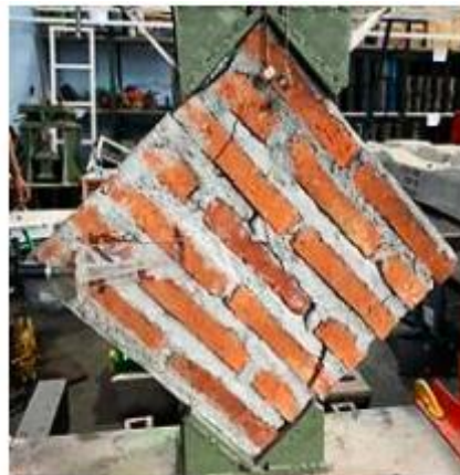
Figure 4: Shear test specimens for DG 03
