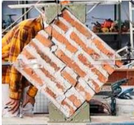
Figure 2: Shear test specimens for DG 01
