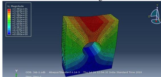
Figure 6: Compressive strength test in Abaqus simulia
