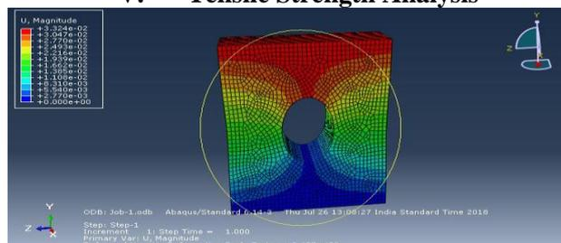
Figure 8: Tensile Strength Test at 20KN Load
