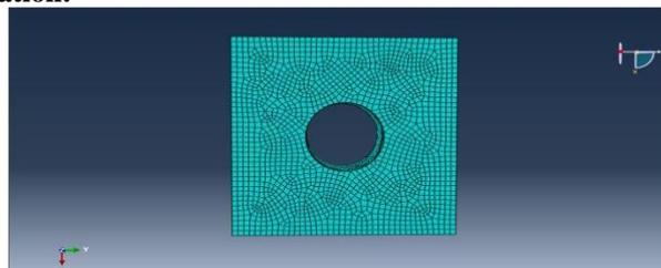
Figure 3: Meshing Applied to Steel Foam Model and Points Generated (22490)
