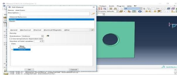
Figure2: Editing Steel Foam material Properties in Abaqus Simulia
