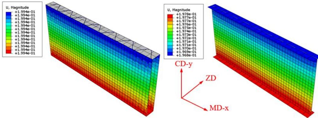
Figure 7. Deformation of the plate after the vertical collision of a 3D model and 2D model
