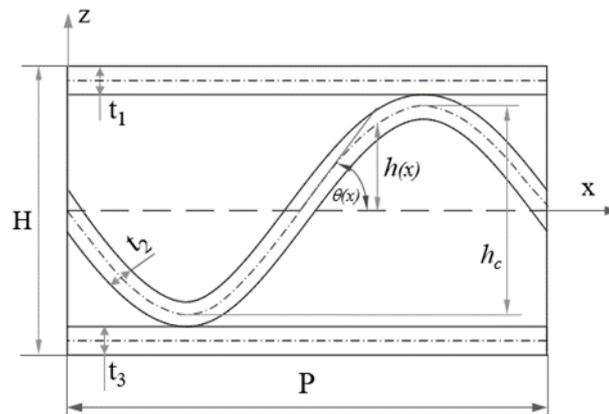
Figure 5. Representative elements of corrugated core sandwich panels
