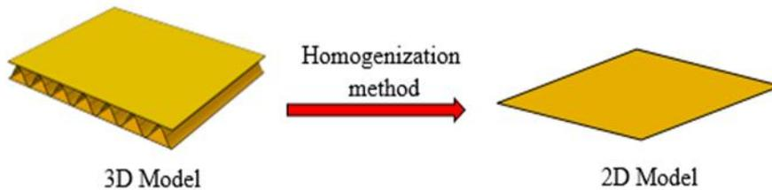
Figure 4. Homogenization method
