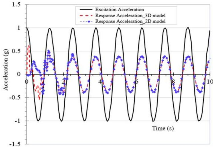
Figure 10. Excited acceleration on the beam in MD direction and response of the two models
