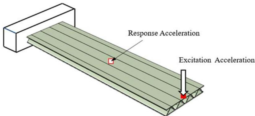
Figure 9. Experimental model simulation of response acceleration measurement.
