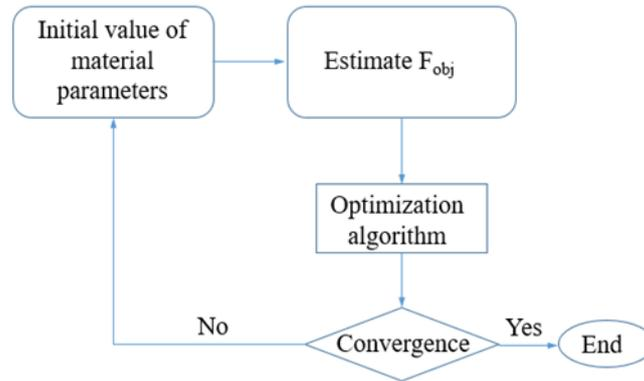
Figure 3. Reverse engineering of paper material parameters
