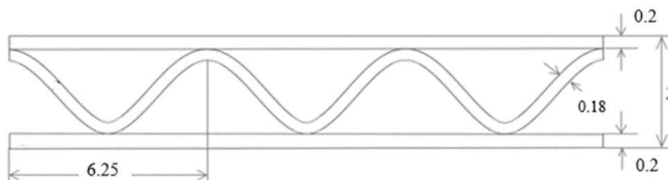
Figure 2. Geometric dimensions of corrugated cardboard type B
