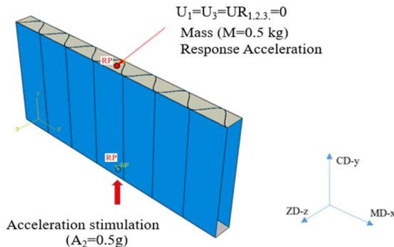
Figure 6. Sandwich panel subjected to vertical impact in the CD direction
