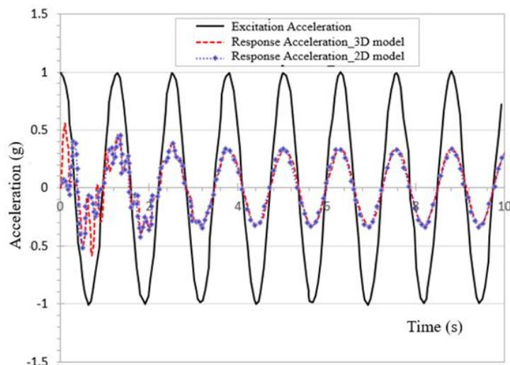
Figure 11. Excited acceleration on the beam in the CD direction and responses of the two models
