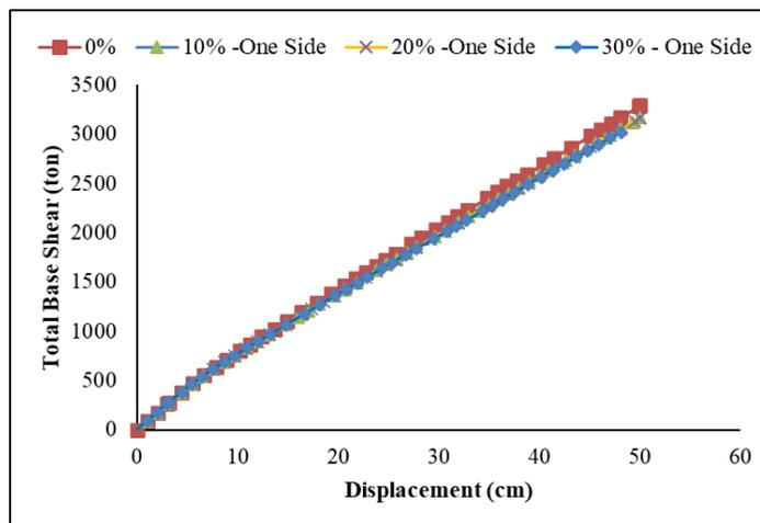
Fig. 12. Load-displacement curves of “One side corrosion” scenario.
