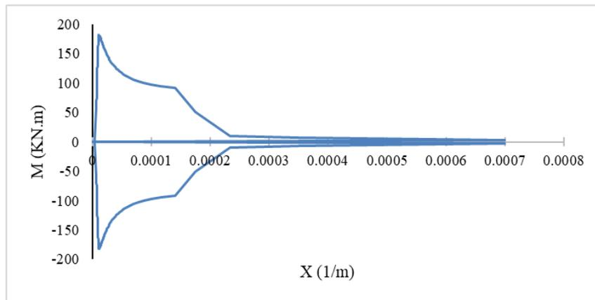
Fig. 9: Curvature-Bending Moment relationships for RC column-30% corrosion.
