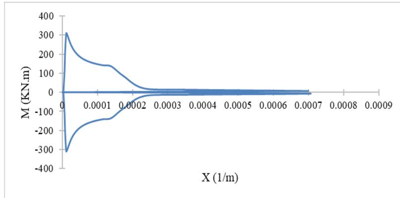
Fig. 7: Curvature-Bending Moment relationships for RC column -10% corrosion.
