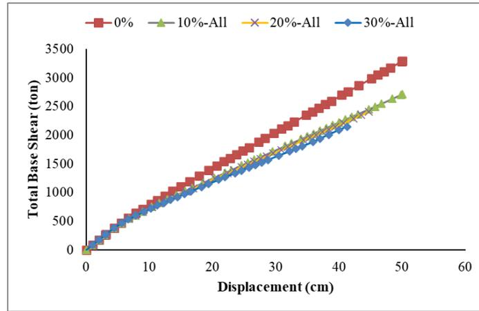
Fig. 11. Load-displacement curves of “All corrosion” scenario.
