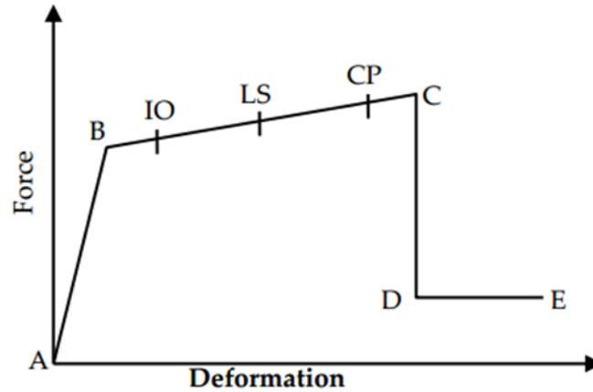
Fig. 10. Force-deformation relationship of a plastic hinge
