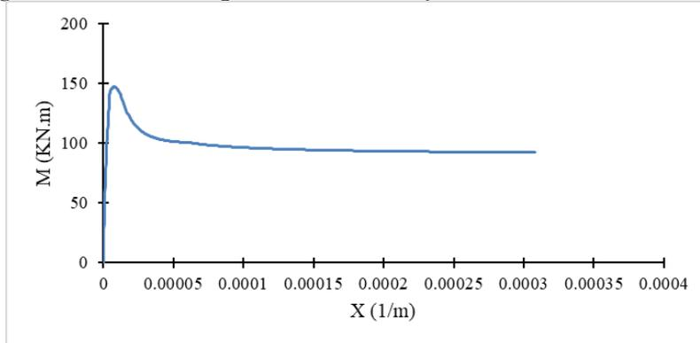
Fig. 4: Curvature-Bending Moment relationships for RC beam - 20% corrosion.
