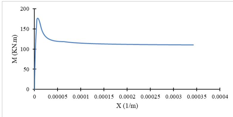
Fig. 3: Curvature-Bending Moment relationships for RC beam - 10% corrosion.
