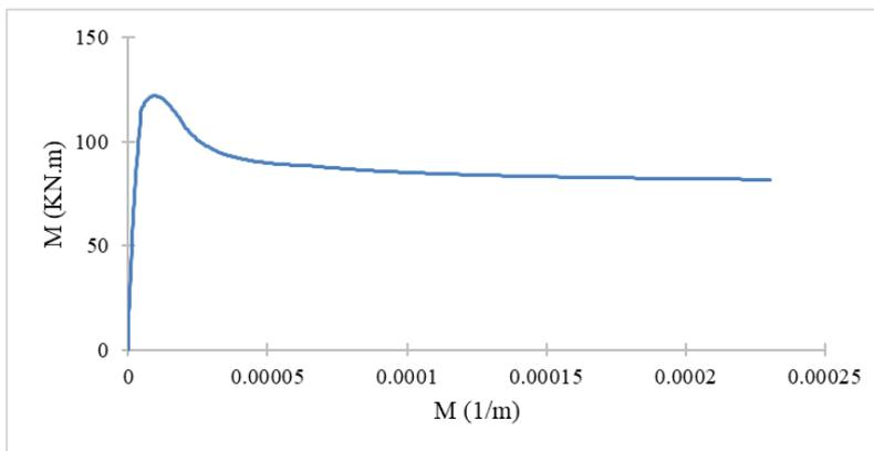
Fig. 5: Curvature-Bending Moment relationships for RC beam - 30% corrosion.
