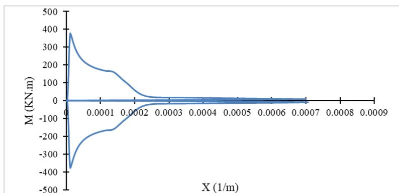
Fig. 6: Curvature-Bending Moment relationships for RC column - 0% corrosion.
