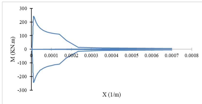
Fig. 8: Curvature-Bending Moment relationships for RC column -20% corrosion.
