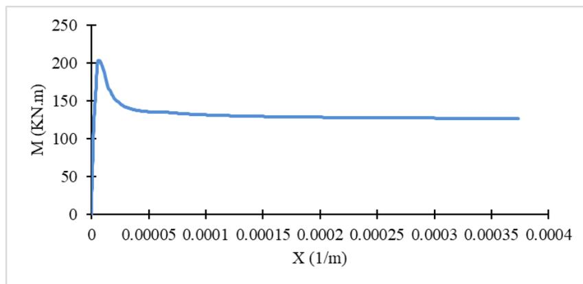
**Fig. 2:** Curvature-Bending Moment relationships for RC beam - 0% corrosion.
