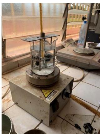
**Figure 2: Softening Point test apparatus**
