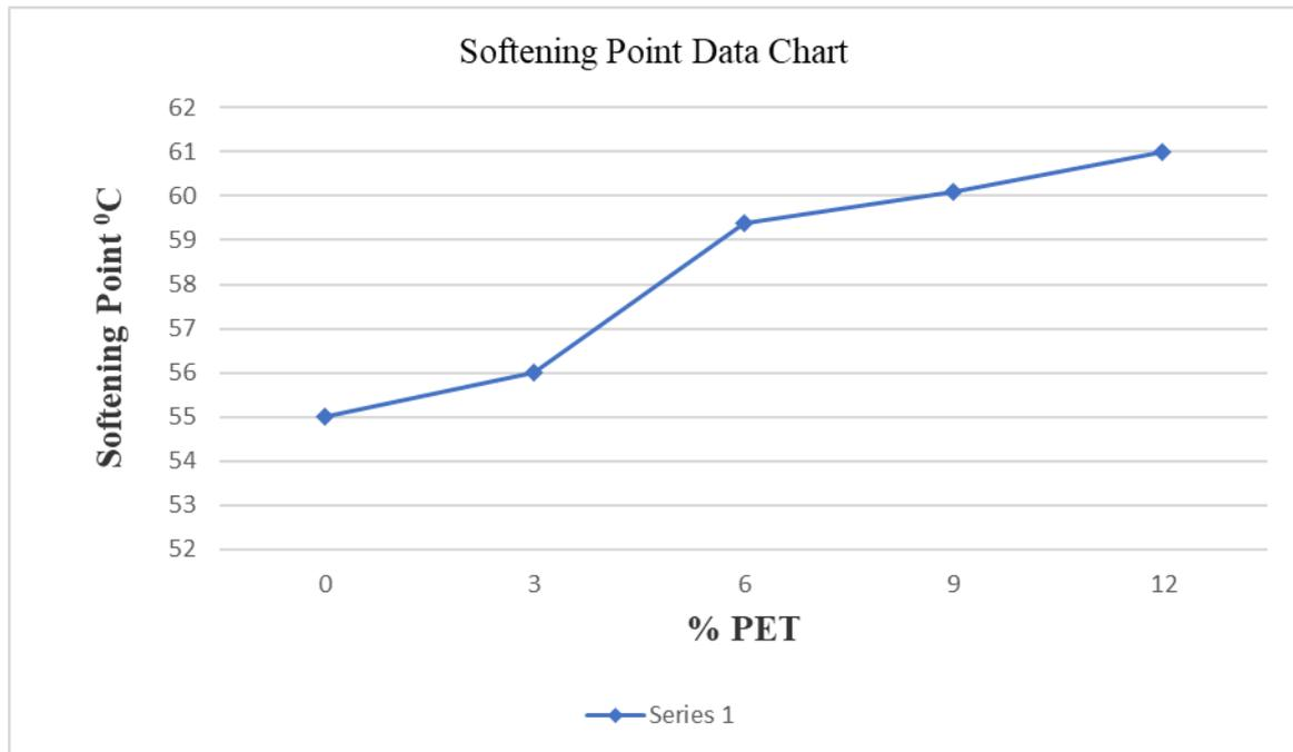
Figure 6: Graphical Illustration for Comparative Softening point results
