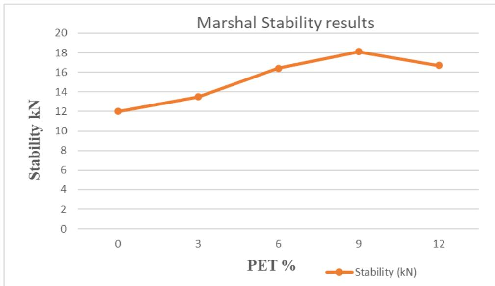
**Figure 9 Graph of Marshal test results**
